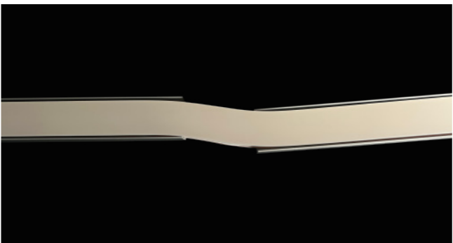
PCB fracture caused by profile misalignment, vertical hanging load, or incorrect installation results in partial dark segments.
