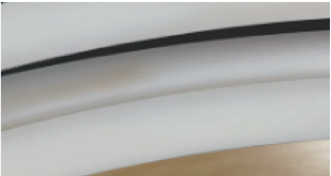
Yellowing of products after prolonged outdoor exposure.
