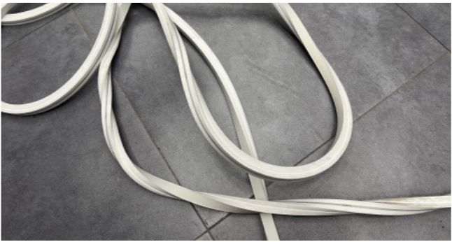
Large reels of neon flex may twist during installation, causing LED failures.
